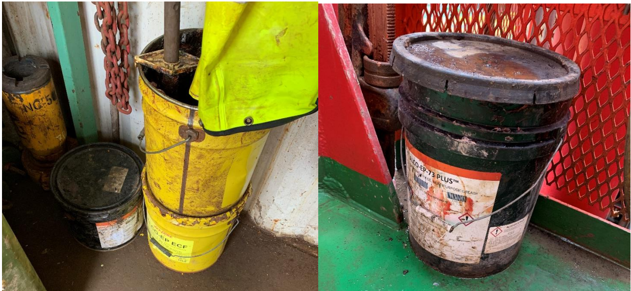
Figure 0-15: Jet-Lube Alco-EP ECF on BOP roof (left) and Jet-Lube Alco EP-73 on drill floor (right)
